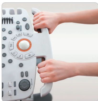
Lifting control panel
